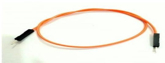
**Gambar 2.5** Kabel Jumper Male to Male
