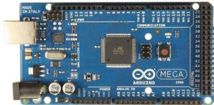
**Gambar 2.1** Papan Arduino Mega
